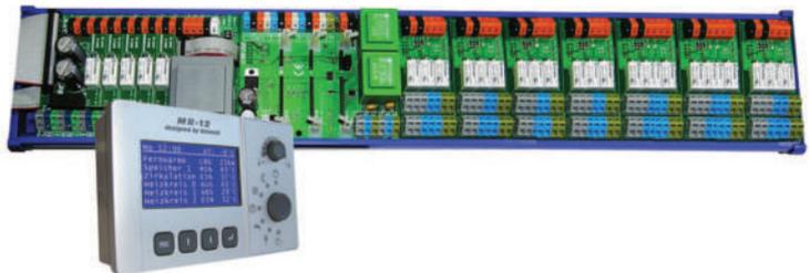
The first heating circuit can also be configured as a charging module circuit for the boiler.
