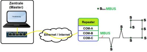
COM-B = CM08-TCP module (Wiznet) or CM06-TCP module (Tibbo)
