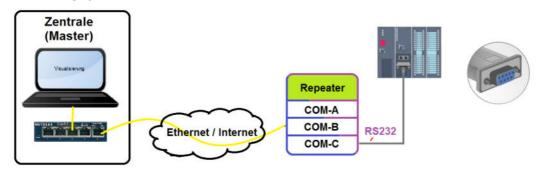
COM-B = CM08-TCP module (Wiznet) or CM06-TCP module (Tibbo) COM-C = RS232
