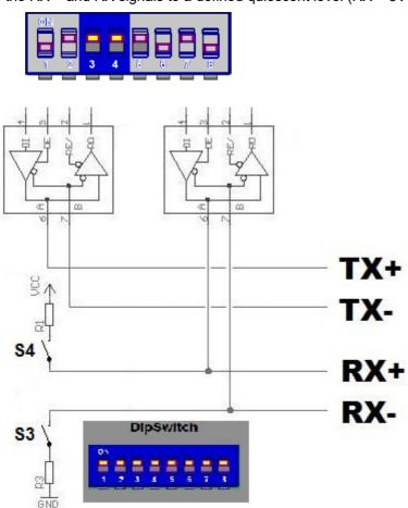
Termination = OFF is required if other interfaces are used that do not need or are not allowed to use termination such as: MBUS.
