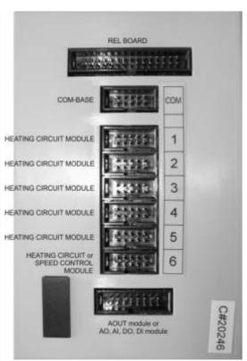
The MR07-PLC is an electronic control device for flush mounting.
